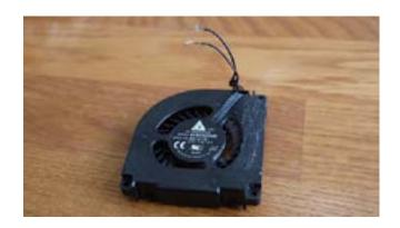
Make sure to know what is + and what is ground on the fan and mark it up with a marker. Twist the cables togheter. Then use "heat shrink tubes" to secure the connection.
