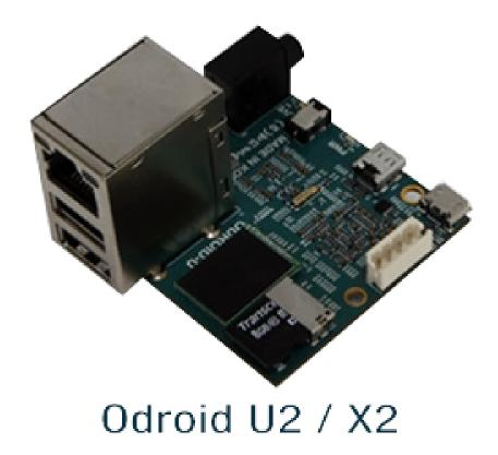
The ODROID U2 is a tricky piece of hardware as console output is not a given. Ideally, when purchasing an ODROID, you should also get a USB UART cable, used for serial debugging of the boot process. Saying this, these machines are (at this time) some of the most impressive in terms of size, horsepower and memory availability.
